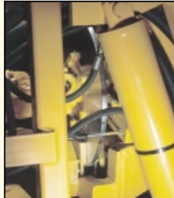
Attention to safety is evident by the driveline brake and LIFELINE® safety rotation shut-off. The driveline brake stops rotation instantly when the LIFELINE® is tripped - a tug of a cable shuts off the drill.
