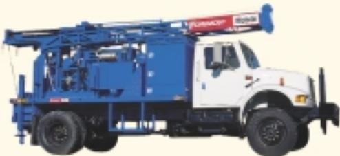
The B-59 driveline is the heart of this rig's exceptional performance. The fully-reversing Clark power shift transmission is equipped with 3 speeds forward and reverse. Combined with our field-proven 2-speed right angle drive, the B-59 delivers a total of 6 speeds to efficiently address all types of drilling conditions.
